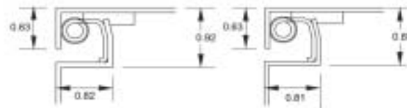
Cross Section of 14 Gauge Body & Door
